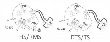
It is possible to set the fan operating time on potentiometer by using a screwdriver in fans with electrical control system (TS, HS and RMS version).
