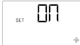
Fig. 5-16 Ventilation function is on
