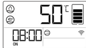
Fig.5-10 Start interface of timer ECO function
