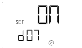
Fig.5-11 Display of sterilization cycle
