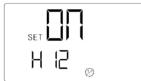
Fig.5-12 Display of sterilization start time
